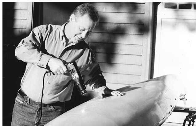
A dent can be removed by applying heat.
